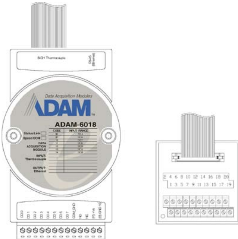
Figure 4.5: ADAM-6018 8-ch Thermocouple Input
