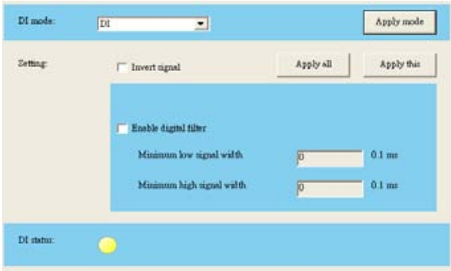
Figure 5.14: Individual Channel Configuration: DI
